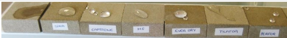
Sin tratar Sikaguard 917W Capstone ST200 Protect Guard MG Ultra Ever dry Filafob TECNADIS PRS PERFORMANCE
